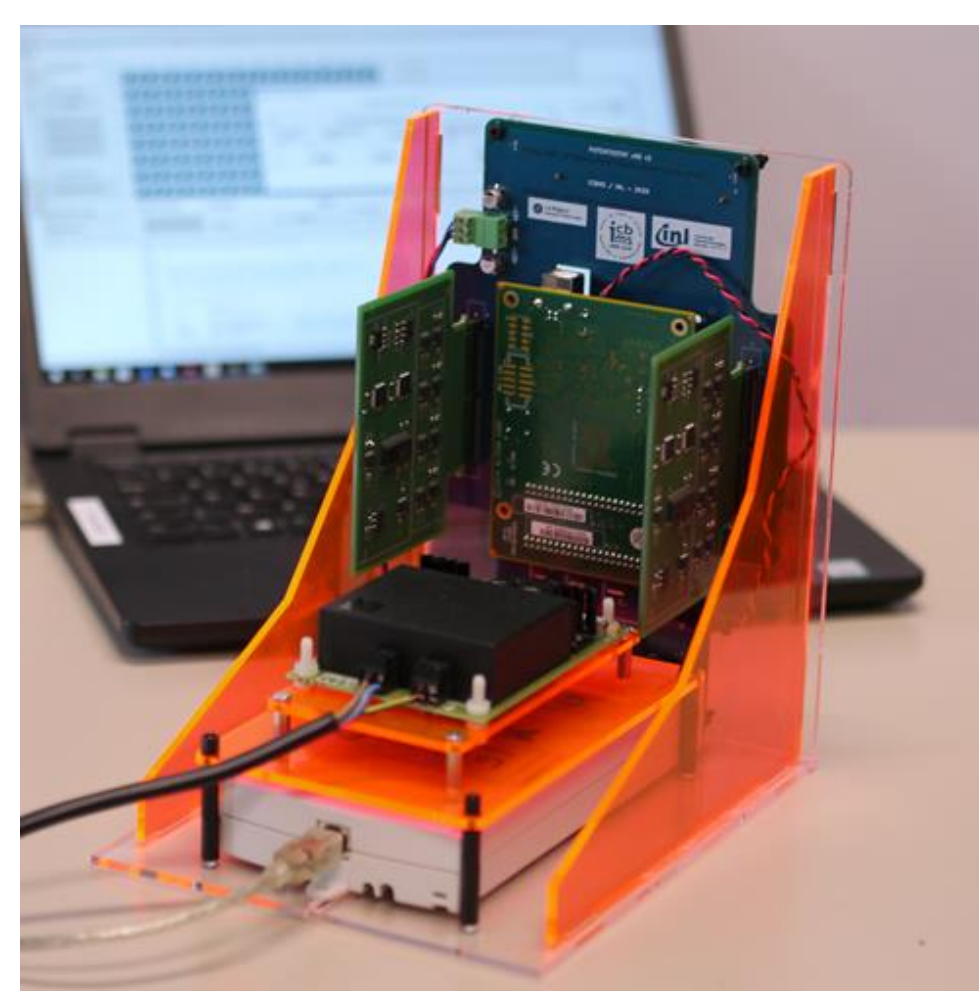
Fig. 1. New IPA device developed by INL. IPA is performed on 96 multiplexed electrodes screen printed on a PCB. Working electrodes are made of carbon and counter/ref are Ag/AgCl electrodes.
